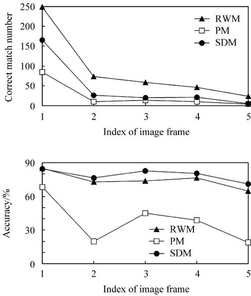
Fig.2 Curves of correct match number vs accuracy for three algorithms: comparison of results for boat sequence with scale and rotation changes.
