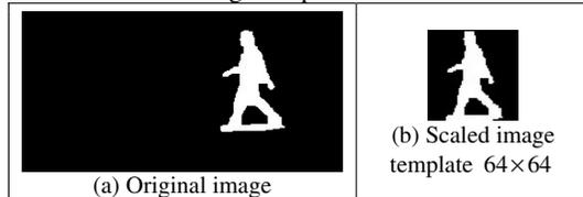
Figure 2. Scaled image template from segmented object.
