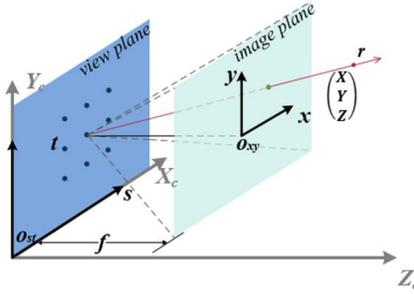
Figure 1. Two-parallel plane model for light field.
