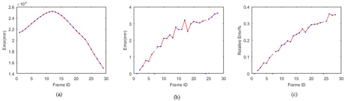
Figure 3. Depth and ray re-projection error map on desk data. (a) depth estimation error; (b) ray re-projection absolute error; (c) ray re-projection relative error.
