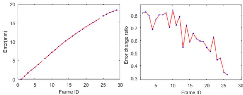
Figure 4. Pose estimation error on the desk data. (a) absolute error ; (b) the error change ratio.
